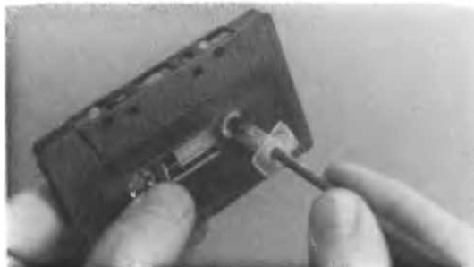
FIG. 10—MANUALLY WINDING A CASSETTE WITH A HOME-MADE TOOL
