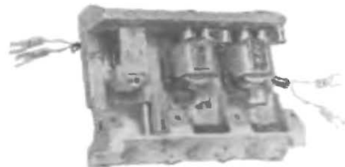
Fig. 4. The three heads are mounted in a complete subassembly.
