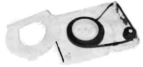
Fig. 4. Same cartridge as shown in Fig. , except with tape guiding disc removed.
