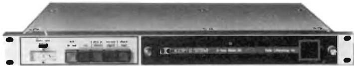
Fig. 7 —Slim, elegant, technically precise, one section of the Dolby A system as used by professional recording bodies throughout the world. Having had the chance to “rip one to bits,” I can vouch for its engineering excellence.
