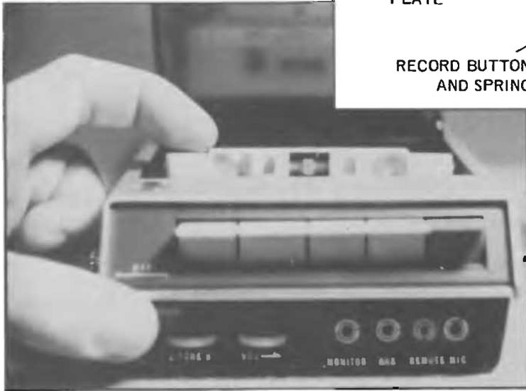
Fig. 2 —With cassette partly ejected and the tape run through to its leader, the pressure pad and spring and the cutaway portions of the cassette are visible.
