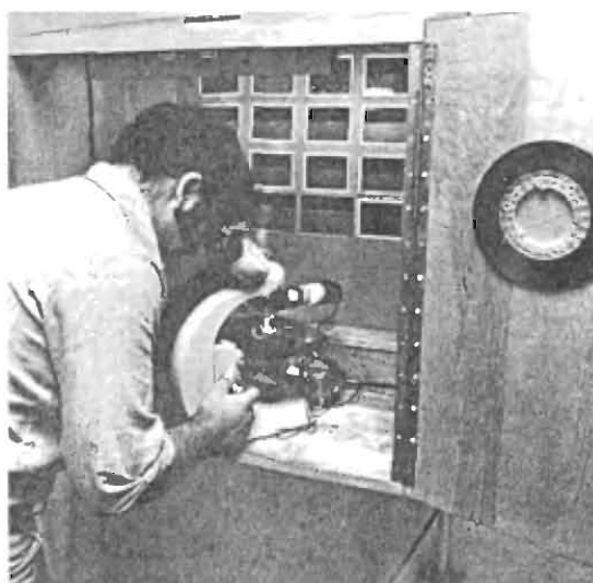
Fig. 2—In slitter operation, tape is unwound from the web (1), transported through blades (2), with slit tape drawn past guides (3), and wound onto pancakes on the far side of the machine. An operator monitors the web during this operation.
