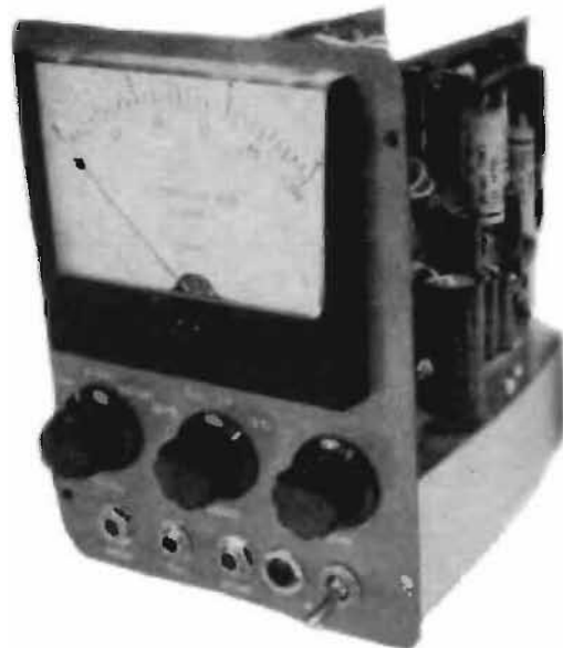
Fig. 1. The completed flutter meter with its protective case removed.
