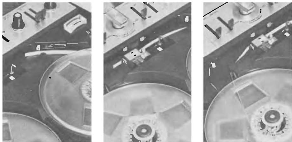
Fig. 1—Automation has come to reel-to-reel tape recorders, including automatic threading. Ampex, Bell & Howell, and Sony Superscope are among manufacturers offering this luxury. Below, is a Bell and Howell Autoload® recorder which, on pressing a lever, activates a blower that lifts tape from the supply reel, carries it under the tape lifter, up toward the takeup reel, and drawn around the reel hub, whereupon the blower shuts off automatically. (Stop-action, strobe-light photography was used here.)
