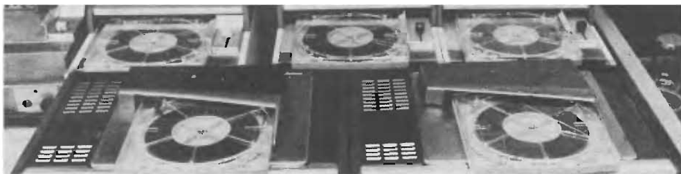
Fig. 2. Tape-punishing setup at 3M testing laboratory in St. Paul. Tapes are fashioned into continuous loops and are run 24 hours a day, giving wear equivalent to 100 years of normal use without appreciable change in performance of tapes. (Photo courtesy 3M.)
