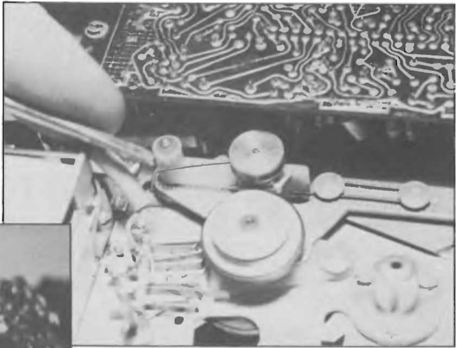
Fig. 9 —Fast-wind action depends on two pulleys and the exact setting of the spring indicated by the screwdriver.
