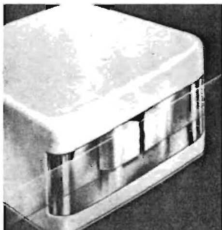
Fig. 1. Erosion of the gap of a tape head due to abrasive action of the tape.
