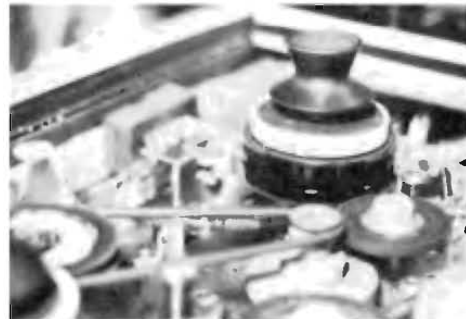
Fig. 7—Sony clutches are efficient, with simple fast-wind action by the heavy-tired idler seen at the right locking motor pulley drive directly to both upper and lower sections of clutch.
