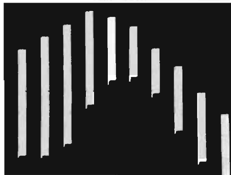
Fig. 2—Range of octave-band maximum levels during a portion of a recording of Mussorgsky's "Night on Bald Mountain."
