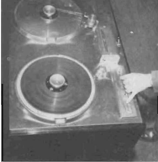
Fig. 1 (left). Top view of professional-type recorder (Ampex). The tape feeds from the loaded supply reel at the left past a tape guide which automatically actuates a motor switch. The control panel is shown below the supply reel, with the magnetic head assembly to its right. The drive capstan and pressure roller are at the right of the head assembly, with the take-up reel above. Fig. 2 (right). Motors and brake-drum assembly of the same machine.
