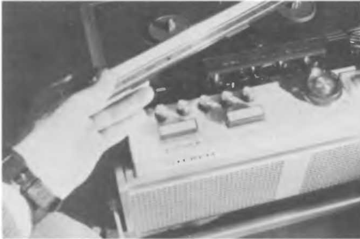
Fig. 7 —Accessibility is half the battle! The front trim of this Grundig deck lifts away completely to allow free access to the heads.
