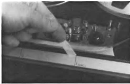
FIG. 7—REBURNISHING, ON A NONMAGNETIC SURFACE
