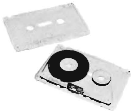
Fig. 6. The Philips cassette with cover removed. This is a 4-track cartridge, using tape 0.15 in. wide in a reel-to-reel configuration, permitting play in either direction.
