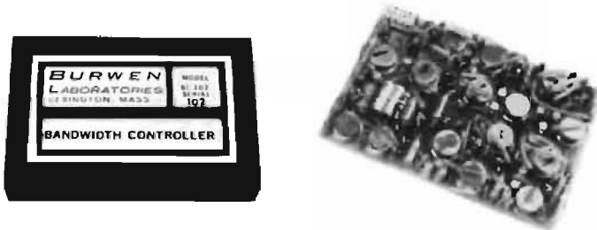
Fig. 5—A high performance module incorporating 15 operational amplifiers.
