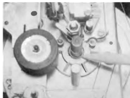
Fig. 4 —Do not overlook the upper bearing of the flywheel capstan when cleaning around the deck. Accumulated oxide at this point can quickly lead to head wear and erratic running.
