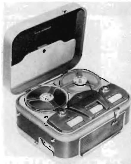
Fig. 1. A tape machine with provision for stereo playback and monophonic recording. (Norelco)
