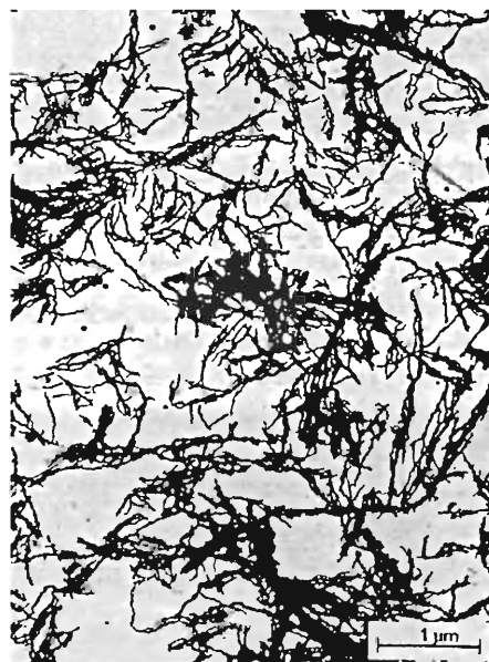
Fig. 3 — Particles used in TDK metal-particle tape.
